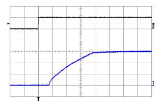
Fig. 6.0V.10: Turn-on transient at full rated load current (resistive) plus 10,000μF at Vin = 24V, triggered via ON/OFF pin. Top trace: ON/OFF signal (5 V/div.). Bottom trace: output voltage (2 V/div.). Time scale: 2 ms/div.
