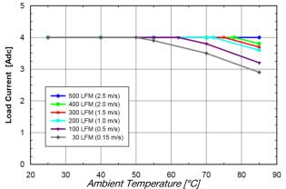
Fig. 12V.4: Available load current vs. ambient temperature and airflow rates for SQ24S04120 converter mounted horizontally with Vin = 24V, air flowing from pin 3 to pin 1 and maximum FET temperature ≤ 120°C.
