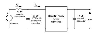
Fig. 2.0V.14: Test setup for measuring input reflected ripple currents, ic and is.
