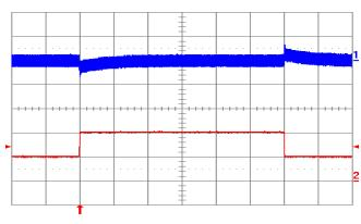
Fig. 12V.11: Output voltage response to load current step-change (1A – 2A – 1A) at Vin = 24V. Top trace: output voltage (200 mV/div.). Bottom trace: load current (1 A/div.). Current slew rate: 0.1 A/μs. Co = 1 μF ceramic. Time scale: 0.5 ms/div.
