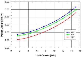
Fig. 1.8V.7: Power dissipation vs. load current and input voltage for SQ24T/S15018 converter mounted vertically with air flowing from pin 3 to pin 1 at a rate of 300 LFM (1.5 m/s) and Ta =  $25^{\circ}$ C.
