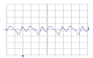
Fig. 1.0V.13: Output voltage ripple (20 mV/div.) at full rated load current into a resistive load with Co = 10 μF tantalum + 1uF ceramic and Vin = 24 V. Time scale: 1 μs/div.
