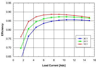
Fig. 2.5V.5: Efficiency vs. load current and input voltage for SQ24T/S15025 converter mounted vertically with air flowing from pin 3 to pin 1 at a rate of 300 LFM (1.5 m/s) and Ta = 25°C.
