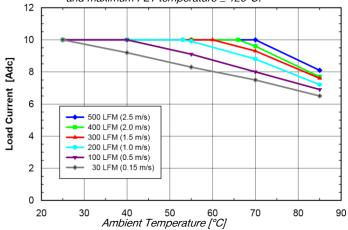
Fig. 5.0V.4: Available load current vs. ambient temperature and airflow rates for SQ24S10050 converter mounted horizontally with Vin = 24V, air flowing from pin 3 to pin 1 and maximum FET temperature ≤ 120°C.
