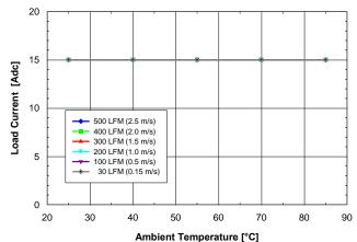
Fig. 1.5V.4: Available load current vs. ambient temperature and airflow rates for SQ24S15015 converter mounted horizontally with Vin = 24V, air flowing from pin 3 to pin 1 and maximum FET temperature ≤ 120°C.
