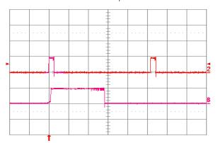
Fig. 2.0V.18: Load current (top trace, 20 A/div., 20 ms/div.) into a 10 m $\Omega$  short circuit during restart, at Vin = 24V. Bottom trace (20 A/div., 2 ms/div.) is an expansion of the on-time portion of the top trace.
