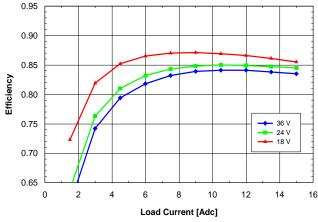
Fig. 1.8V.5: Efficiency vs. load current and input voltage for SQ24T/S15018 converter mounted vertically with air flowing from pin 3 to pin 1 at a rate of 300 LFM (1.5 m/s) and Ta = 25°C.
