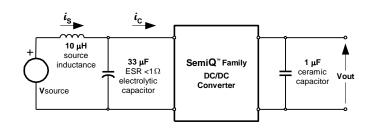
Fig. 6.0V.14: Test setup for measuring input reflected ripple currents, ic and is.
