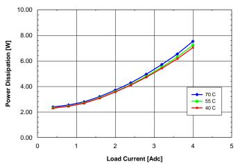
Fig. 12V.8: Power dissipation vs. load current and ambient temperature for SQ24T/S04120 converter mounted vertically with Vin = 24V and air flowing from pin 3 to pin 1 at a rate of 200 LFM (1.0 m/s).
