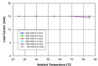
Fig. 1.8V.4: Available load current vs. ambient temperature and airflow rates for SQ24S15018 converter mounted horizontally with Vin = 24V, air flowing from pin 3 to pin 1 and maximum FET temperature ≤ 120°C.
