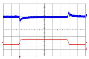
Fig. 1.8V.11: Output voltage response to load current step-change (3.75A – 7.5A – 3.75A) at Vin = 24V. Top trace: output voltage (100 mV/div.). Bottom trace: load current (5 A/div.). Current slew rate: 0.1 A/μs. Co = 1 μF ceramic. Time scale: 0.2 ms/div.
