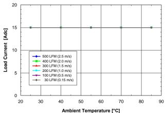
Fig. 1.2V.4: Available load current vs. ambient temperature and airflow rates for SQ24S15012 converter mounted horizontally with Vin = 24V, air flowing from pin 3 to pin 1 and maximum FET temperature ≤ 120°C.
