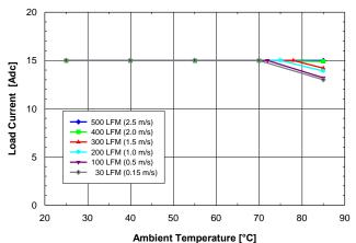
Fig. 2.0V.1: Available load current vs. ambient air temperature and airflow rates for SQ24T15020 converter with B height pins mounted vertically with Vin = 24V, air flowing from pin 3 to pin 1
