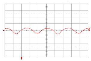
Fig. 1.2V.15: Input reflected ripple current, ic (100 mA/div.), measured at input terminals at full rated load current and Vin = 24V. Refer to Fig. 1.2V.14 for test setup. Time scale: 1  $\mu$ s/div.
