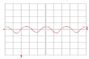
Fig. 1.8V.15: Input reflected ripple current, ic (100 mA/div.), measured at input terminals at full rated load current and Vin = 24V. Refer to Fig. 1.8V.14 for test setup. Time scale: 1  $\mu$ s/div.
