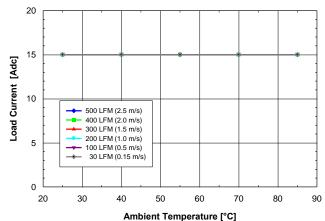
Fig. 1.0V.4: Available load current vs. ambient temperature and airflow rates for SQ24S15010 converter mounted horizontally with Vin = 24V, air flowing from pin 3 to pin 1 and maximum FET temperature ≤ 120°C.
