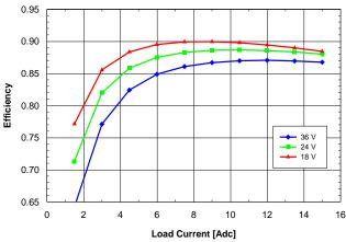
Fig. 3.3V.5: Efficiency vs. load current and input voltage for SQ24T/S15033 converter mounted vertically with air flowing from pin 3 to pin 1 at a rate of 300 LFM (1.5 m/s) and Ta = 25°C.
