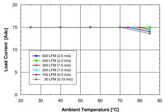
Fig. 1.8V.3: Available load current vs. ambient temperature and airflow rates for SQ24S15018 converter mounted vertically with Vin = 24V, air flowing from pin 3 to pin 1 and maximum FET temperature  $\leq$  120°C.
