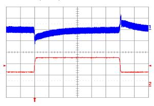
Fig. 5.0V.11: Output voltage response to load current step-change (2.5A – 5A – 2.5A) at Vin = 24V. Top trace: output voltage (100 mV/div.). Bottom trace: load current (2 A/div.). Current slew rate: 0.1 A/μs. Co = 1 μF ceramic. Time scale: 0.2 ms/div.
