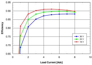
Fig. 6.0V.5: Efficiency vs. load current and input voltage for SQ24T/S08060 converter mounted vertically with air flowing from pin 3 to pin 1 at a rate of 300 LFM (1.5 m/s) and Ta = 25°C.
