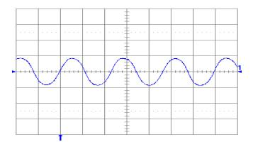
Fig. 12V.13: Output voltage ripple (50 mV/div.) at full rated load current into a resistive load with Co = 10 μF tantalum + 1uF ceramic and Vin = 24 V. Time scale: 1 μs/div.
