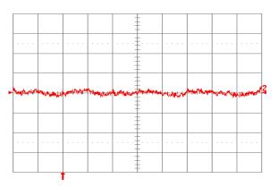
Fig. 6.0V.16: Input reflected ripple current, is (10 mA/div.), measured through 10  $\mu$ H at the source at full rated load current and Vin = 24V. Refer to Fig. 6.0V.14 for test setup. Time scale:  $1\mu$ s/div.
