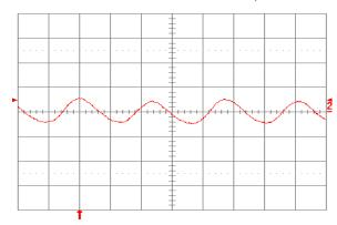
Fig. 3.3V.15: Input reflected ripple current, ic (100 mA/div.), measured at input terminals at full rated load current and Vin = 24V. Refer to Fig. 3.3V.14 for test setup. Time scale: 1  $\mu$ s/div.
