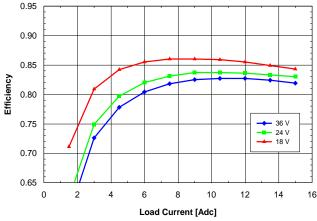
Fig. 1.5V.5: Efficiency vs. load current and input voltage for SQ24T/S15015 converter mounted vertically with air flowing from pin 3 to pin 1 at a rate of 300 LFM (1.5 m/s) and Ta = 25°C.
