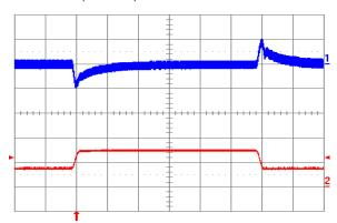
Fig. 1.2V.11: Output voltage response to load current step-change (3.75 A – 7.5 A – 3.75 A) at Vin = 24V. Top trace: output voltage (100 mV/div.). Bottom trace: load current (5 A/div.). Current slew rate: 0.1 A/μs. Co = 1 μF ceramic. Time scale: 0.2 ms/div.
