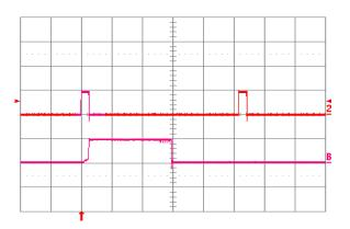
Fig. 1.2V.18: Load current (top trace, 20 A/div., 20 ms/div.) into a 10 m $\Omega$  short circuit during restart, at Vin = 24V. Bottom trace (20 A/div., 2 ms/div.) is an expansion of the on-time portion of the top trace.
