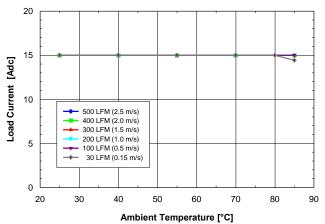
Fig. 1.8V.2: Available load current vs. ambient air temperature and airflow rates for SQ24T15018 converter with B height pins mounted horizontally with Vin = 24V, air flowing from pin 3 to pin 1 and maximum FET temperature ≤ 120°C.
