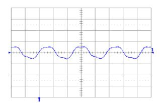
Fig. 6.0V.13: Output voltage ripple (50 mV/div.) at full rated load current into a resistive load with Co = 10 μF tantalum + 1uF ceramic and Vin = 24 V. Time scale: 1 μs/div.
