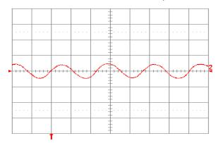
Fig. 2.5V.15: Input reflected ripple current, ic (100 mA/div.), measured at input terminals at full rated load current and Vin = 24V. Refer to Fig. 2.5V.14 for test setup. Time scale: 1  $\mu$ s/div.
