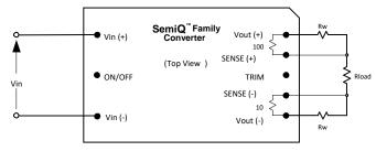
Fig. B: Remote sense circuit configuration.
