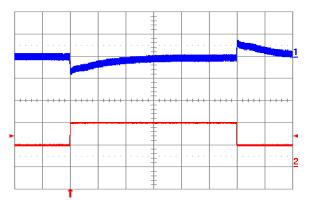
Fig. 6.0V.12: Output voltage response to load current step-change (2A – 4A – 2A) at Vin = 24V. Top trace: output voltage (100mV/div.). Bottom trace: load current (2A/div.). Current slew rate: 5 A/μs. Co = 450 μF tantalum + 1 μF ceramic. Time scale: 0.2 ms/div.
