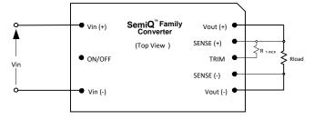
Fig. C: Configuration for increasing output voltage.
