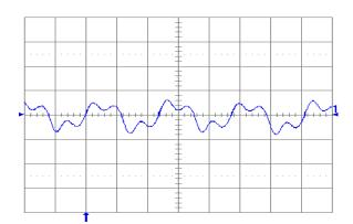
Fig. 2.5V.13: Output voltage ripple (20 mV/div.) at full rated load current into a resistive load with Co = 10 μF tantalum + 1uF ceramic and Vin = 24 V. Time scale: 1 μs/div.
