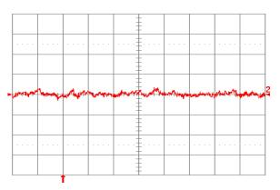
Fig. 1.2V.16: Input reflected ripple current, is (10 mA/div.), measured through 10  $\mu$ H at the source at full rated load current and Vin = 24V. Refer to Fig. 1.2V.14 for test setup. Time scale:  $1\mu$ s/div.
