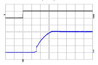
Fig. 1.5V.10: Turn-on transient at full rated load current (resistive) plus 10,000 μF at Vin = 24V, triggered via ON/OFF pin. Top trace: ON/OFF signal (5 V/div.). Bottom trace: output voltage (0.5 V/div.). Time scale: 1 ms/div.
