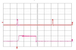
Fig. 3.3V.18: Load current (top trace, 20 A/div., 20 ms/div.) into a 10 m $\Omega$  short circuit during restart, at Vin = 24V. Bottom trace (20 A/div., 1 ms/div.) is an expansion of the on-time portion of the top trace.
