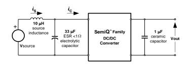
Fig. 3.3V.14: Test setup for measuring input reflected ripple currents, ic and is.
