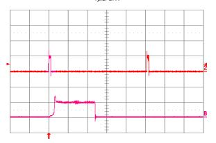
Fig. 2.5V.18: Load current (top trace, 20 A/div., 20 ms/div.) into a 10 m $\Omega$  short circuit during restart, at Vin = 24V. Bottom trace (20 A/div., 1 ms/div.) is an expansion of the on-time portion of the top trace.
