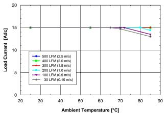
Fig. 2.0V.2: Available load current vs. ambient air temperature and airflow rates for SQ24T15020 converter with B height pins mounted horizontally with Vin = 24V, air flowing from pin 3 to pin 1 and maximum FET temperature ≤ 120°C.
