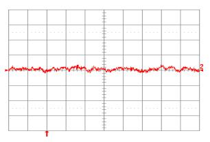
Fig. 1.0V.16: Input reflected ripple current, is (10 mA/div.), measured through 10  $\mu$ H at the source at full rated load current and Vin = 24V. Refer to Fig. 1.0V.14 for test setup. Time scale:  $1\mu$ s/div.
