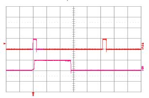
Fig. 1.5V.18: Load current (top trace, 20 A/div., 20 ms/div.) into a 10 m $\Omega$  short circuit during restart, at Vin = 24V. Bottom trace (20 A/div., 2 ms/div.) is an expansion of the on-time portion of the top trace.
