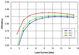
Fig. 2.0V.5: Efficiency vs. load current and input voltage for SQ24T/S15020 converter mounted vertically with air flowing from pin 3 to pin 1 at a rate of 300 LFM (1.5 m/s) and Ta = 25°C.
