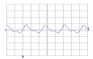
Fig. 3.3V.13: Output voltage ripple (20 mV/div.) at full rated load current into a resistive load with Co = 10 μF tantalum + 1uF ceramic and Vin = 24 V. Time scale: 1 μs/div.
