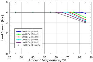
Fig. 12V.3: Available load current vs. ambient temperature and airflow rates for SQ24S04120 converter mounted vertically with Vin = 24V, air flowing from pin 3 to pin 1 and maximum FET temperature ≤ 120°C.
