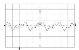
Fig. 2.0V.13: Output voltage ripple (20 mV/div.) at full rated load current into a resistive load with Co = 10 μF tantalum + 1uF ceramic and Vin = 24 V. Time scale: 1 μs/div.
