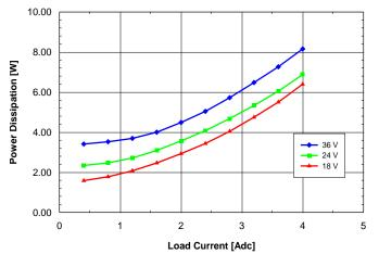
Fig. 12V.7: Power dissipation vs. load current and input voltage for SQ24T/S04120 converter mounted vertically with air flowing from pin 3 to pin 1 at a rate of 300 LFM (1.5 m/s) and Ta =  $25^{\circ}$ C.
