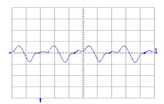
Fig. 1.8V.13: Output voltage ripple (20 mV/div.) at full rated load current into a resistive load with Co = 10 μF tantalum + 1uF ceramic and Vin = 24 V. Time scale: 1 μs/div.
