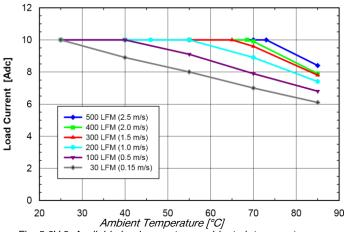
Fig. 5.0V.2: Available load current vs. ambient air temperature and airflow rates for SQ24T10050 converter with B height pins mounted horizontally with Vin = 24V, air flowing from pin 3 to pin 1 and maximum FET temperature ≤ 120°C.
