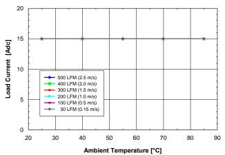
Fig. 1.5V.2: Available load current vs. ambient air temperature and airflow rates for SQ24T15015 converter with B height pins mounted horizontally with Vin = 24V, air flowing from pin 3 to pin 1 and maximum FET temperature ≤ 120°C.
