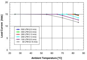
Fig. 2.5V.2: Available load current vs. ambient air temperature and airflow rates for SQ24T15025 converter with B height pins mounted horizontally with Vin = 24V, air flowing from pin 3 to pin 1 and maximum FET temperature ≤ 120°C.
