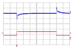
Fig. 1.0V.12: Output voltage response to load current step-change (3.75 A – 7.5 A – 3.75 A) at Vin = 24V. Top trace: output voltage (100 mV/div.). Bottom trace: load current (5 A/div.). Current slew rate: 5 A/ $\mu$ s. Co = 450  $\mu$ F tantalum + 1  $\mu$ F ceramic. Time scale: 0.2 ms/div.
