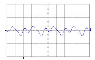
Fig. 1.2V.13: Output voltage ripple (20 mV/div.) at full rated load current into a resistive load with Co = 10 μF tantalum + 1uF ceramic and Vin = 24 V. Time scale: 1 μs/div.
