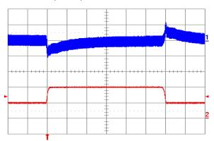
Fig. 6.0V.11: Output voltage response to load current step-change (2A – 4A – 2A) at Vin = 24V. Top trace: output voltage (100mV/div.). Bottom trace: load current (2A/div.). Current slew rate: 0.1 A/μs. Co = 1 μF ceramic. Time scale: 0.2 ms/div.
