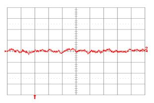
Fig. 5.0V.16: Input reflected ripple current, is (10 mA/div.), measured through 10  $\mu$ H at the source at full rated load current and Vin = 24V. Refer to Fig. 5.0V.14 for test setup. Time scale:  $1\mu$ s/div.
