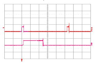
Fig. 6.0V.18: Load current (top trace, 20 A/div., 20 ms/div.) into a 10 m $\Omega$  short circuit during restart, at Vin = 24V. Bottom trace (20 A/div., 2 ms/div.) is an expansion of the on-time portion of the top trace.
