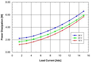
Fig. 2.5V.7: Power dissipation vs. load current and input voltage for SQ24T/S15025 converter mounted vertically with air flowing from pin 3 to pin 1 at a rate of 300 LFM (1.5 m/s) and Ta =  $25^{\circ}$ C.
