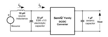
Fig. 1.5V.14: Test setup for measuring input reflected ripple currents, ic and is.
