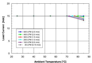
Fig. 2.0V.3: Available load current vs. ambient temperature and airflow rates for SQ24S15020 converter mounted vertically with Vin = 24V, air flowing from pin 3 to pin 1 and maximum FET temperature ≤ 120°C.
