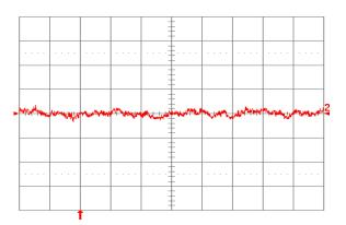
Fig. 2.0V.16: Input reflected ripple current, is (10 mA/div.), measured through 10 μH at the source at full rated load current and Vin = 24V. Refer to Fig. 2.0V.14 for test setup. Time scale: 1μs/div.
