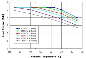
Fig. 8.0V.1: Available load current vs. ambient air temperature and airflow rates for SQ24T05080 converter with D height pins mounted vertically with Vin = 24 V, air flowing from pin 3 to pin 1 and maximum FET temperature ≤ 120°C.
