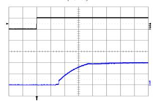
Fig. 2.0V.10: Turn-on transient at full rated load current (resistive) plus 10,000μF at Vin = 24V, triggered via ON/OFF pin. Top trace: ON/OFF signal (5 V/div.). Bottom trace: output voltage (1 V/div.). Time scale: 1 ms/div.
