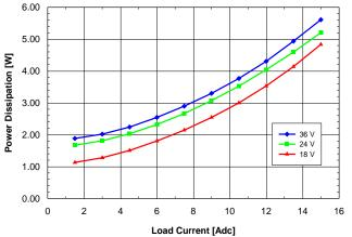
Fig. 2.0V.7: Power dissipation vs. load current and input voltage for SQ24T/S15020 converter mounted vertically with air flowing from pin 3 to pin 1 at a rate of 300 LFM (1.5 m/s) and Ta =  $25^{\circ}$ C.
