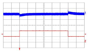
Fig. 12V.12: Output voltage response to load current step-change (1A – 2A – 1A) at Vin = 24V. Top trace: output voltage (200 mV/div.). Bottom trace: load current (1 A/div.). Current slew rate: 5 A/μs. Co = 1 μF ceramic. Time scale: 0.5 ms/div.
