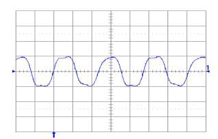
Fig. 5.0V.13: Output voltage ripple (20 mV/div.) at full rated load current into a resistive load with Co = 10 μF tantalum + 1uF ceramic and Vin = 24 V. Time scale: 1 μs/div.
