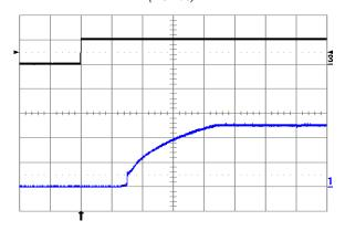
Fig. 2.5V.10: Turn-on transient at full rated load current (resistive) plus 10,000 μF at Vin = 24V, triggered via ON/OFF pin. Top trace: ON/OFF signal (5 V/div.). Bottom trace: output voltage (1 V/div.). Time scale: 1 ms/div.
