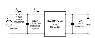
Fig. 1.0V.14: Test setup for measuring input reflected ripple currents, ic and is.
