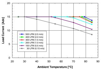
Fig. 3.3V.2: Available load current vs. ambient air temperature and airflow rates for SQ24T15033 converter with B height pins mounted horizontally with Vin = 24V, air flowing from pin 3 to pin 1 and maximum FET temperature ≤ 120°C.
