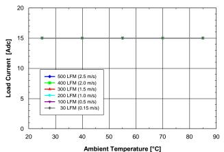
Fig. 1.0V.3: Available load current vs. ambient temperature and airflow rates for SQ24S15010 converter mounted vertically with Vin = 24V, air flowing from pin 3 to pin 1 and maximum FET temperature ≤ 120°C.
