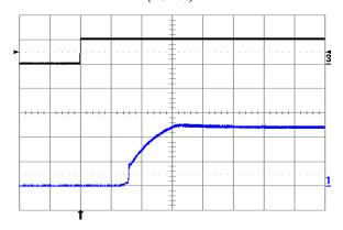
Fig. 1.2V.10: Turn-on transient at full rated load current (resistive) plus 10,000 μF at Vin = 24V, triggered via ON/OFF pin. Top trace: ON/OFF signal (5 V/div.). Bottom trace: output voltage (0.5 V/div.). Time scale: 1 ms/div.
