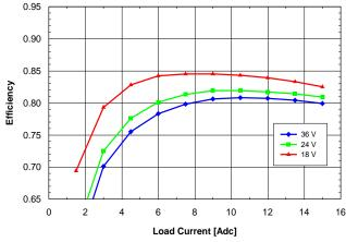
Fig. 1.2V.5: Efficiency vs. load current and input voltage for SQ24T/S15012 converter mounted vertically with air flowing from pin 3 to pin 1 at a rate of 300 LFM (1.5 m/s) and Ta = 25°C.
