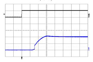
Fig. 1.0V.10: Turn-on transient at full rated load current (resistive) plus 10,000μF at Vin = 24V, triggered via ON/OFF pin. Top trace: ON/OFF signal (5 V/div.). Bottom trace: output voltage (0.5 V/div.). Time scale: 1 ms/div.
