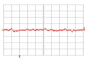
Fig. 1.8V.16: Input reflected ripple current, is (10 mA/div.), measured through 10  $\mu$ H at the source at full rated load current and Vin = 24V. Refer to Fig. 1.8V.14 for test setup. Time scale:  $1\mu$ s/div.
