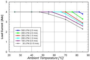
Fig. 12V.1: Available load current vs. ambient air temperature and airflow rates for SQ24T04120 converter with B height pins mounted vertically with Vin = 24V, air flowing from pin 3 to pin 1 and maximum FET temperature ≤ 120°C.
