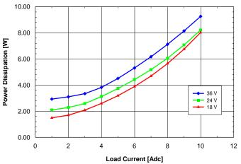
Fig. 5.0V.7: Power dissipation vs. load current and input voltage for SQ24T/S10050 converter mounted vertically with air flowing from pin 3 to pin 1 at a rate of 300 LFM (1.5 m/s) and Ta =  $25^{\circ}$ C.
