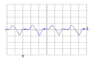
Fig. 1.5V.13: Output voltage ripple (20 mV/div.) at full rated load current into a resistive load with Co = 10 μF tantalum + 1uF ceramic and Vin = 24 V. Time scale: 1 μs/div.
