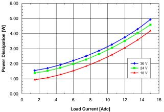
Fig. 1.5V.7: Power dissipation vs. load current and input voltage for SQ24T/S15015 converter mounted vertically with air flowing from pin 3 to pin 1 at a rate of 300 LFM (1.5 m/s) and Ta =  $25^{\circ}$ C.
