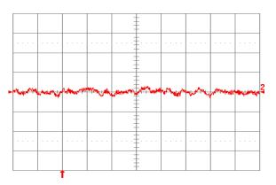
Fig. 1.5V.16: Input reflected ripple current, is (10 mA/div.), measured through 10  $\mu$ H at the source at full rated load current and Vin = 24V. Refer to Fig. 1.5V.14 for test setup. Time scale:  $1\mu$ s/div.
