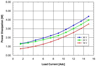
Fig. 1.0V.7: Power dissipation vs. load current and input voltage for SQ24T/S15010 converter mounted vertically with air flowing from pin 3 to pin 1 at a rate of 300 LFM (1.5 m/s) and Ta =  $25^{\circ}$ C.
