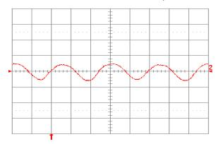
Fig. 2.0V.15: Input reflected ripple current, ic (100 mA/div.), measured at input terminals at full rated load current and Vin = 24V. Refer to Fig. 2.0V.14 for test setup. Time scale: 1 µs/div.
