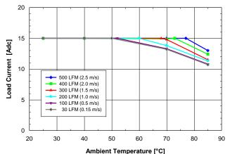
Fig. 3.3V.3: Available load current vs. ambient temperature and airflow rates for SQ24S15033 converter mounted vertically with Vin = 24V, air flowing from pin 3 to pin 1 and maximum FET temperature ≤ 120°C.
