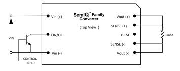
Fig. A: Circuit configuration for ON/OFF function.
