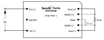
Fig. D: Configuration for decreasing output voltage.
