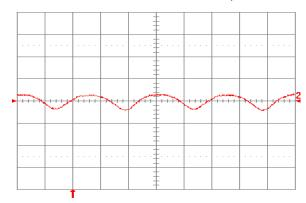
Fig. 1.0V.15: Input reflected ripple current, ic (100 mA/div.), measured at input terminals at full rated load current and Vin = 24V. Refer to Fig. 1.0V.14 for test setup. Time scale: 1  $\mu$ s/div.
