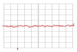
Fig. 3.3V.16: Input reflected ripple current, is (10 mA/div.), measured through 10  $\mu$ H at the source at full rated load current and Vin = 24V. Refer to Fig. 3.3V.14 for test setup. Time scale:  $1\mu$ s/div.
