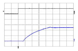
Fig. 5.0V.10: Turn-on transient at full rated load current (resistive) plus 10,000 μF at Vin = 24V, triggered via ON/OFF pin. Top trace: ON/OFF signal (5 V/div.). Bottom trace: output voltage (2 V/div.). Time scale: 2 ms/div.
