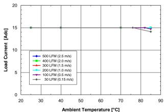
Fig. 1.5V.3: Available load current vs. ambient temperature and airflow rates for SQ24S15015 converter mounted vertically with Vin = 24V, air flowing from pin 3 to pin 1 and maximum FET temperature ≤ 120°C.
