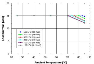
Fig. 2.5V.1: Available load current vs. ambient air temperature and airflow rates for SQ24T15025 converter with B height pins mounted vertically with Vin = 24V, air flowing from pin 3 to pin 1 and maximum FET temperature ≤ 120°C.
