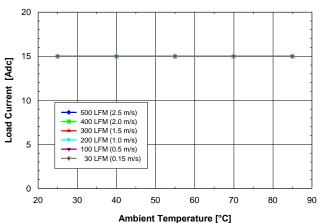
Fig. 1.2V.2: Available load current vs. ambient air temperature and airflow rates for SQ24T15012 converter with B height pins mounted horizontally with Vin = 24V, air flowing from pin 3 to pin 1 and maximum FET temperature ≤ 120°C.
