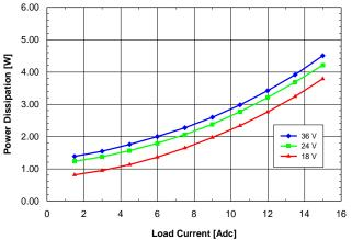
Fig. 1.2V.7: Power dissipation vs. load current and input voltage for SQ24T/S15012 converter mounted vertically with air flowing from pin 3 to pin 1 at a rate of 300 LFM (1.5 m/s) and Ta =  $25^{\circ}$ C.
