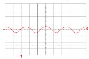
Fig. 1.5V.15: Input reflected ripple current, ic (100 mA/div.), measured at input terminals at full rated load current and Vin = 24V. Refer to Fig. 1.5V.14 for test setup. Time scale: 1  $\mu$ s/div.
