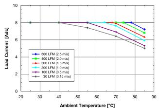
Fig. 6.0V.1: Available load current vs. ambient air temperature and airflow rates for SQ24T08060 converter with B height pins mounted vertically with Vin = 24V, air flowing from pin 3 to pin 1 and maximum FET temperature ≤ 120°C.
