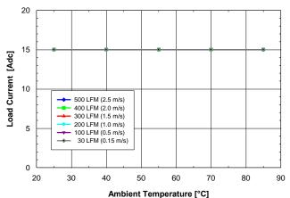
Fig. 1.2V.3: Available load current vs. ambient temperature and airflow rates for SQ24S15012 converter mounted vertically with Vin = 24V, air flowing from pin 3 to pin 1 and maximum FET temperature ≤ 120°C.
