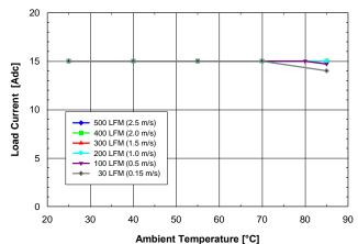
Fig. 2.0V.4: Available load current vs. ambient temperature and airflow rates for SQ24S15020 converter mounted horizontally with Vin = 24V, air flowing from pin 3 to pin 1 and maximum FET temperature ≤ 120°C.
