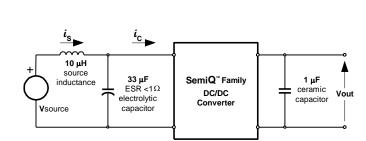
Fig. 1.2V.14: Test setup for measuring input reflected ripple currents, ic and is.
