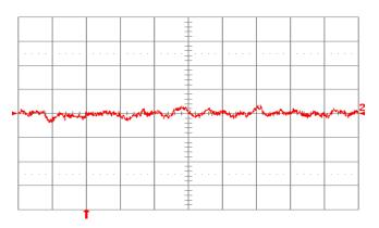
Fig. 12V.16: Input reflected ripple current, is (10 mA/div.), measured through  $10\mu$ H at the source at full rated load current and Vin = 24V. Refer to Fig. 12V.14 for test setup. Time scale:  $1\mu$ s/div.
