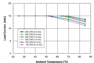
Fig. 3.3V.4: Available load current vs. ambient temperature and airflow rates for SQ24S15033 converter mounted horizontally with Vin = 24V, air flowing from pin 3 to pin 1 and maximum FET temperature < 120°C.
