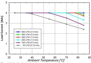
Fig. 12V.2: Available load current vs. ambient air temperature and airflow rates for SQ24T04120 converter with B height pins mounted horizontally with Vin = 24V, air flowing from pin 3 to pin 1 and maximum FET temperature ≤ 120°C.
