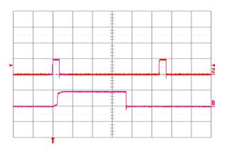
Fig. 1.0V.18: Load current (top trace, 20 A/div., 20 ms/div.) into a 10 m $\Omega$  short circuit during restart, at Vin = 24V. Bottom trace (20 A/div., 2 ms/div.) is an expansion of the on-time portion of the top trace.
