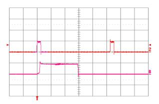
Fig. 1.8V.18: Load current (top trace, 20 A/div., 20 ms/div.) into a 10 m $\Omega$  short circuit during restart, at Vin = 24V. Bottom trace (20 A/div., 2 ms/div.) is an expansion of the on-time portion of the top trace.
