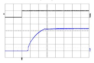
Fig. 3.3V.10: Turn-on transient at full rated load current (resistive) plus 10,000 μF at Vin = 24V, triggered via ON/OFF pin. Top trace: ON/OFF signal (5 V/div.). Bottom trace: output voltage (1 V/div.). Time scale: 2 ms/div.
