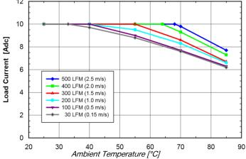
Fig. 5.0V.3: Available load current vs. ambient temperature and airflow rates for SQ24S10050 converter mounted vertically with Vin = 24V, air flowing from pin 3 to pin 1 and maximum FET temperature ≤ 120°C..
