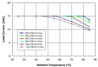
Fig. 3.3V.1: Available load current vs. ambient air temperature and airflow rates for SQ24T15033 converter with B height pins mounted vertically with Vin = 24V, air flowing from pin 3 to pin 1 and maximum FET temperature ≤ 120°C.
