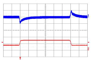
Fig. 1.5V.11: Output voltage response to load current step-change (3.75 A – 7.5 A – 3.75 A) at Vin = 24V. Top trace: output voltage (100 mV/div.). Bottom trace: load current (5 A/div.). Current slew rate: 0.1 A/μs. Co = 1 μF ceramic. Time scale: 0.2 ms/div.
