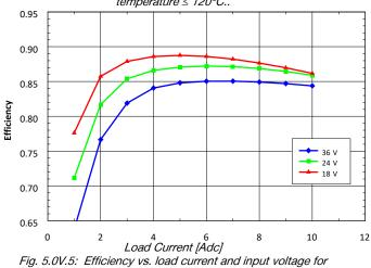
Fig. 5.0V.5: Efficiency vs. load current and input voltage for SQ24T/S10050 converter mounted vertically with air flowing from pin 3 to pin 1 at a rate of 300 LFM (1.5 m/s) and Ta = 25°C.
