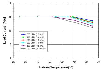
Fig. 2.5V.4: Available load current vs. ambient temperature and airflow rates for SQ24S15025 converter mounted horizontally with Vin = 24V, air flowing from pin 3 to pin 1 and maximum FET temperature ≤ 120°C.
