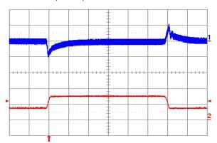
Fig. 2.0V.11: Output voltage response to load current step-change (3.75A – 7.5A – 3.75A) at Vin = 24V. Top trace: output voltage (100 mV/div.). Bottom trace: load current (5 A/div.). Current slew rate: 0.1 A/μs. Co = 1 μF ceramic. Time scale: 0.2 ms/div.
