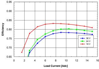
Fig. 1.0V.5: Efficiency vs. load current and input voltage for SQ24T/S15010 converter mounted vertically with air flowing from pin 3 to pin 1 at a rate of 300 LFM (1.5 m/s) and Ta = 25°C.
