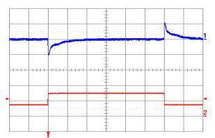
Fig. 3.3V.12: Output voltage response to load current step-change (3.75A – 7.5A – 3.75A) at Vin = 24V. Top trace: output voltage (100 mV/div.). Bottom trace: load current (5 A/div.). Current slew rate: 5 A/μs. Co = 450 μF tantalum + 1 μF ceramic. Time scale: 0.2 ms/div.
