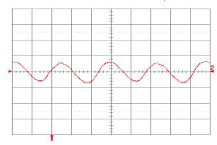
Fig. 6.0V.15: Input reflected ripple current, ic (100 mA/div.), measured at input terminals at full rated load current and Vin = 24V. Refer to Fig. 6.0V.14 for test setup. Time scale: 1  $\mu$ s/div.
