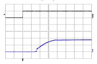
Fig. 1.8V.10: Turn-on transient at full rated load current (resistive) plus 10,000μF at Vin = 24V, triggered via ON/OFF pin. Top trace: ON/OFF signal (5 V/div.). Bottom trace: output voltage (1 V/div.). Time scale: 1 ms/div.
