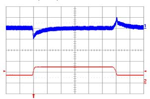
Fig. 3.3V.11: Output voltage response to load current step-change (3.75A – 7.5A – 3.75A) at Vin = 24V. Top trace: output voltage (100 mV/div.). Bottom trace: load current (5 A/div.). Current slew rate: 0.1 A/μs. Co = 1 μF ceramic. Time scale: 0.2 ms/div.
