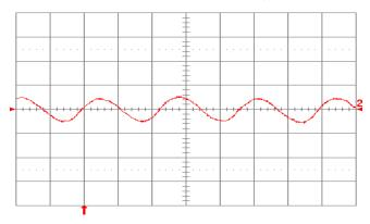
Fig. 12V.15: Input reflected ripple current, ic (100 mA/div.), measured at input terminals at full rated load current and Vin = 24V. Refer to Fig. 12V.14 for test setup. Time scale: 1  $\mu$ s/div.
