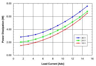
Fig. 3.3V.7: Power dissipation vs. load current and input voltage for SQ24T/S15033 converter mounted vertically with air flowing from pin 3 to pin 1 at a rate of 300 LFM (1.5 m/s) and Ta =  $25^{\circ}$ C.
