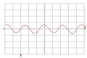
Fig. 5.0V.15: Input reflected ripple current, ic (100 mA/div.), measured at input terminals at full rated load current and Vin = 24V. Refer to Fig. 5.0V.14 for test setup. Time scale: 1  $\mu$ s/div.
