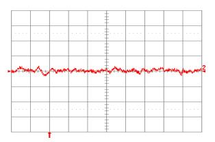
Fig. 2.5V.16: Input reflected ripple current, is (10 mA/div.), measured through 10  $\mu$ H at the source at full rated load current and Vin = 24V. Refer to Fig. 2.5V.14 for test setup. Time scale:  $1\mu$ s/div.
