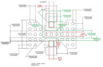
NOTE: If possible, use copper filled vias underneath pin 3 for better thermals; otherwise, use vias that are plated through, filled and plated over.
