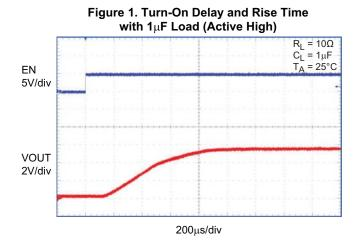
Figure 3. Turn-On Delay and Rise Time
