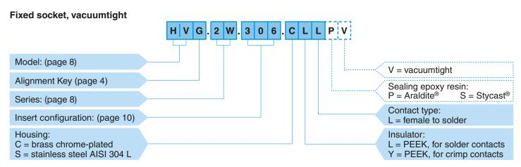
**HVG.2W.306.CLLPV** = fixed socket, nut fixing, key (G), 2W series, multipole type with 6 contacts, outer shell in chrome-plated brass, PEEK insulator, female solder contacts, potted with Araldite® epoxy resin, vacuumtight.
