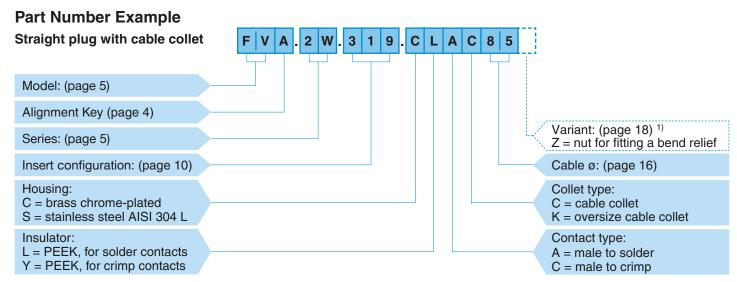
**FVA.2W.319.CLAC85** = straight plug with key (A), 2W series, multipole type with 19 contacts, outer shell in chrome-plated brass, PEEK insulator, male solder contacts, C type collet for 8.5 mm diameter cable.
