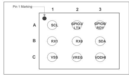
Figure 1.2 IQS624 pin-out (WLCSP-9 package top view; markings may differ) Table 1.2 WLCSP-9 pin-out description
