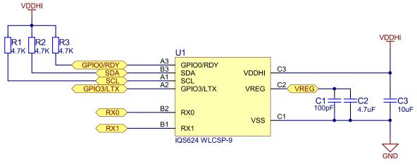
Figure 1.4 IQS624 WLCSP-9 reference schematic
