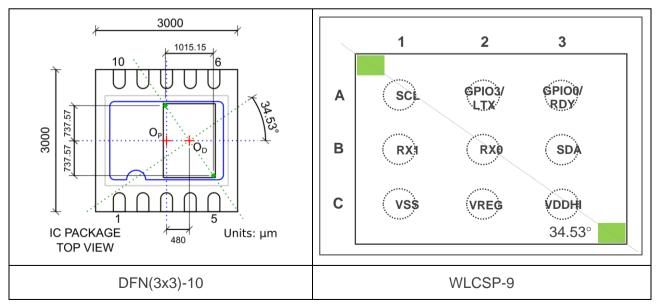
Figure 13.1 Figure 13-1 - Technical Drawing showing DIE placement within the package. The Hall-Plates are shown as the two green pads in the corners of the DIE. Package axis and hall-plate axis are also shown.
