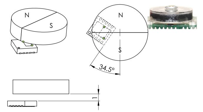
Figure 13.3 Figure 13-2 Magnet's postion relative to IC with on-axis orientation Figure 13.4 Table 13-1 Typical specifications of on-axis magnet position
