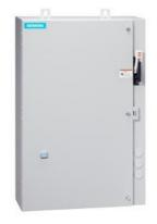
Non-reversing motor starter, Size 2, Three phase full voltage, Solid-state overload relay, OLR amp range 13-52A, 110V 50Hz / 120V 60Hz coil, Combination type, 60A fusible disconnect, 60A/600V fuse clip, Encl NEMA type 4X 304 S-Steel, Water/dust tight noncorrosive, Extra-wide enclosure
