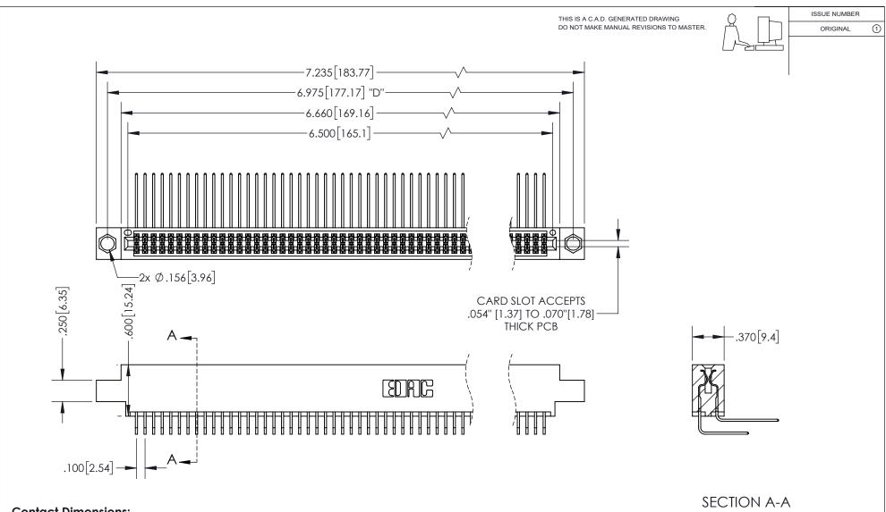
**Contact Dimensions:** 559-90 Degree Bend (Code 541 Contacts) See Sheet 2 for Contact Code 555, 556, 558, 559, 560 Dimensions
