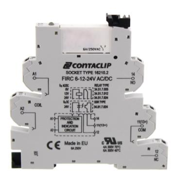
Interface-Relay-Compact (IRC) Complete, Consisting of base FIRC... with Push-In connection and pluggable miniature relay with power contact, Mounting type: Mounting rail TS 35, 1 CO contact, Input voltage: 24 VAC/DC
