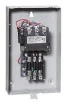
Non-reversing motor starter, Size 2 1/2, Three phase full voltage, Amb. compensate bimetal OLR, Contactor amp rating 60A, 24VAC 50-60Hz coil, Non-combination type, Enclosure type 1, Indoor general purpose use
