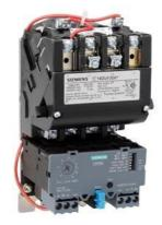
Non-reversing motor starter Size 1 Three phase full voltage Solid-state overload relay OLRelay amp range 10-40a 24Vdc coil Combination type No enclosure
