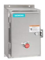
Non-reversing motor starter, Size 0, Three phase full voltage, Solid-state overload relay, OLR amp range 3-12A, Non-combination type, Encl. type 4X 304 S. Steel, Water/dust tight noncorrosive, Standard width enclosure
