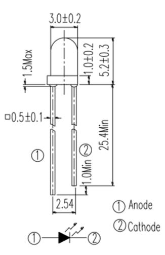
Note: Tolerances unless dimensions ±0.25mm
