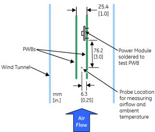
Figure 13. Thermal Test Setup.
