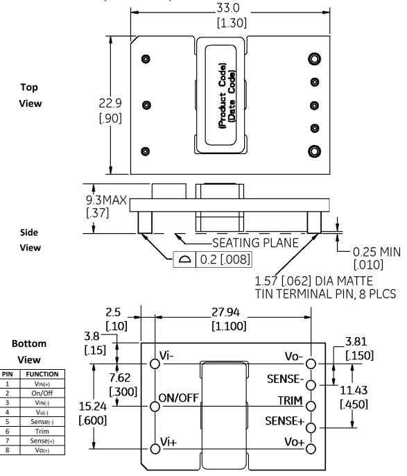
18-75Vdc Input; 5.0Vdc, 8A/10A Output
