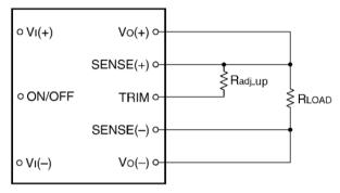
Figure 12. Circuit Configuration to Increase Output Voltage.
