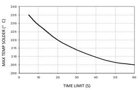
Figure 21. Time Limit,  $T_{\text{lim}}\text{, Curve Above 205}^{\circ}\text{C Reflow}$  .
