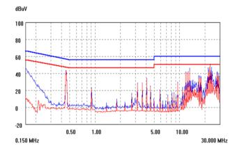
Figure 18. EMC signature using above filter, KHHD010A0.
