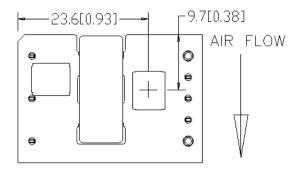
Figure 16. T<sub>ref</sub> Temperature Measurement Location.
