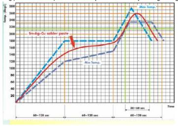
Fig 2. Infrared soldering profile
