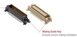
**Lineup Combination** Receptacle 52885 55091 53625 53647 53649 53627 Series No. Circuits 20 to 240 20 to 200 20 to 240 20 to 160 30 to 140 20 to 200 Mated Height (mm) 6.00 to 10.00 6.00 7.00 8.00 9.00 10.00 Receptacle Plug 52901 55091 53625 53647 53649 53627 Series No. 20 to 200 Circuits 20 to 200 20 to 200 20 to 200 20 to 160 30 to 140 Mated Height (mm) 12.00 to 16.00 14.00 15.00 16.00 12.00 13.00
