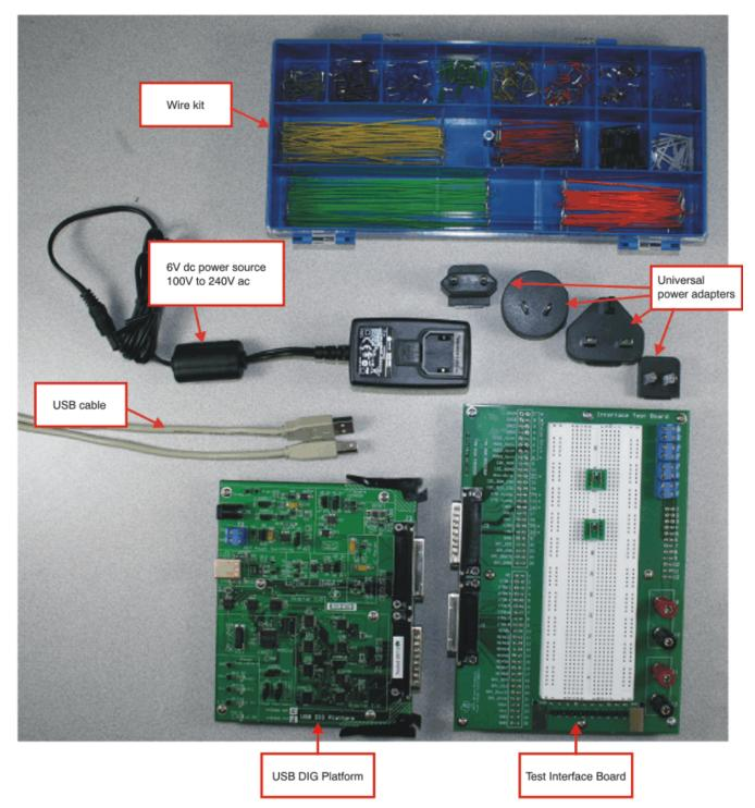
Figure 1. Hardware Included with the Serial-Bus-EVM
