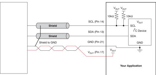
Figure 10. Cable Design with Shield (Eliminates Capacitive Coupling Between Cables)
