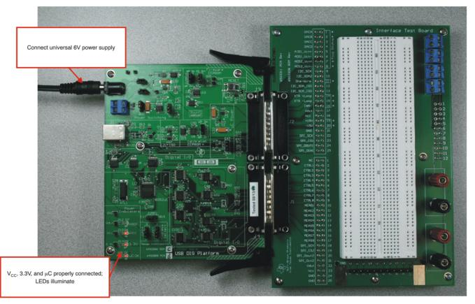
Figure 4. Connecting Power to the EVM
