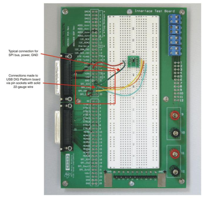
Figure 6. Interface Test Board Signal Connections
