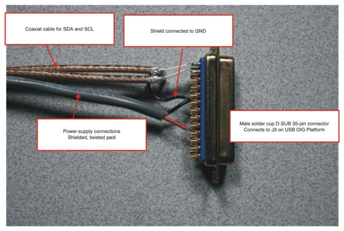
Figure 11. Shielded Cable Build on Solder Cup D-Sub
