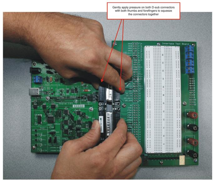
Figure 3. Connecting the Two EVM PCBs
