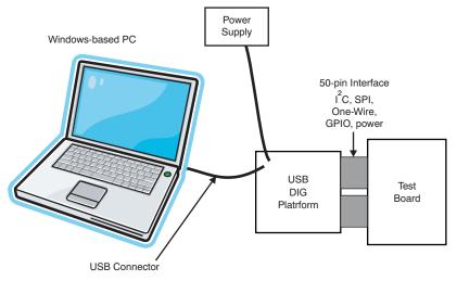
Figure 2. USB DIG Platform Hardware Setup
