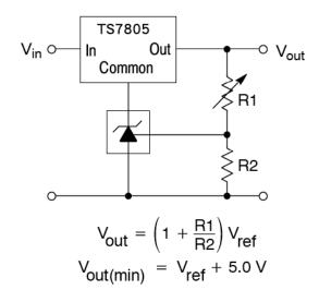
Figure 2. Output Control for Three Terminal Fixed Regulator
