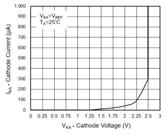
Figure 18. Cathode Current vs. Cathode Voltage
