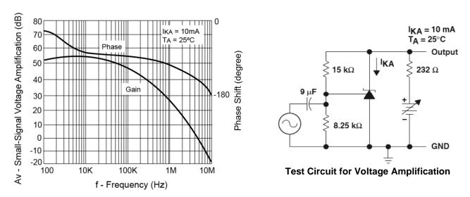
Figure 12. Small-Signal Voltage Gain and Phase Shift vs. Frequency
