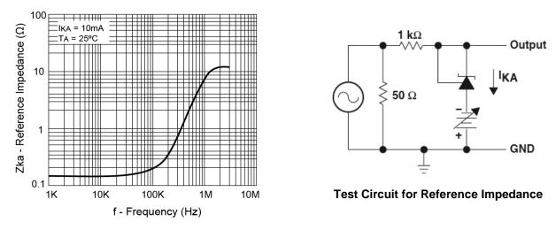
Figure 13. Reference Impedance vs. Frequency
