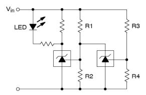
L.E.D. indicator is 'ON' when V<sub>in</sub> is between the upper and lower limits,
