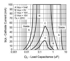
The areas under the curves represent conditions that may cause the device to oscillate. For curves B, C, and D, R2 and V+ were adjusted to establish the initial VKA and IKA conditions with CL=0. VBATT and CL then were adjusted to determine the ranges of stability.
