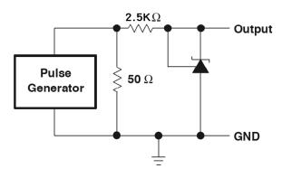
Test Circuit for Pulse Response, I<sub>K</sub>=1mA
