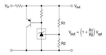
**Figure 4. High Current Shunt Regulator**
