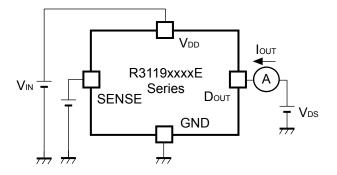
Nch Driver Output Current Test Circuit
