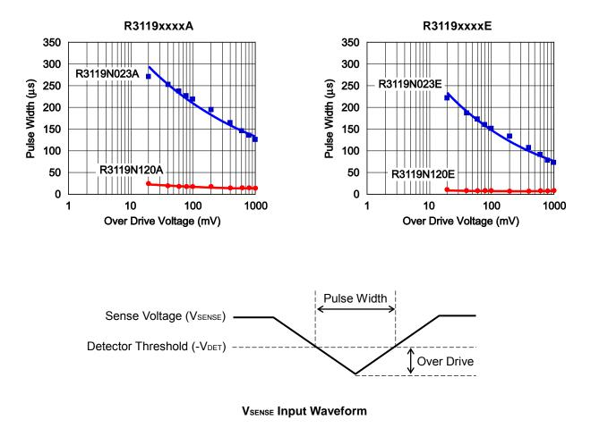
This graph shows the maximum pulse conditions to keep the released voltage. If the pulse with larger amplitude or wider width than the graph above, is input to the  $V_{DD}$  pin (R3119xxxxA) or to the SENSE pin (R3119xxxxE), the reset signal may be output.
