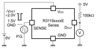
**Output Delay Time Test Circuit**
