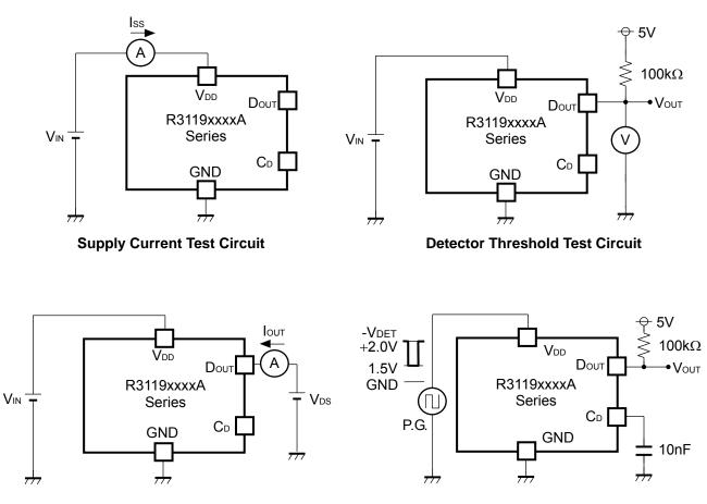
Nch Driver Output Current Test Circuit
