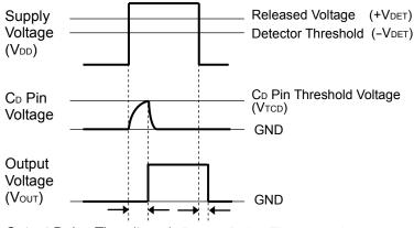
Output Delay Time (tdelay) Detect Delay Time (treset)
