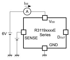
**Supply Current Test Circuit**
