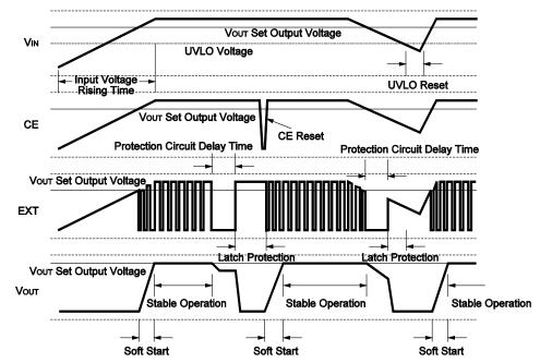
The timing chart shown above describes the changing process of input voltage rising, stable operating, operating with large current, reset with CE pin, stable operating, input voltage falling, input voltage recovering, and stable operating.
