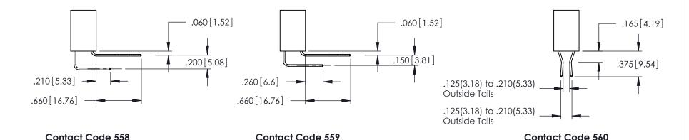
INSULATOR MATERIAL: THERMOPLASTIC POLYESTER, UL 94V-0 CONTACT MATERIAL; COPPER, NICKEL, TIN ALLOY CA-725
