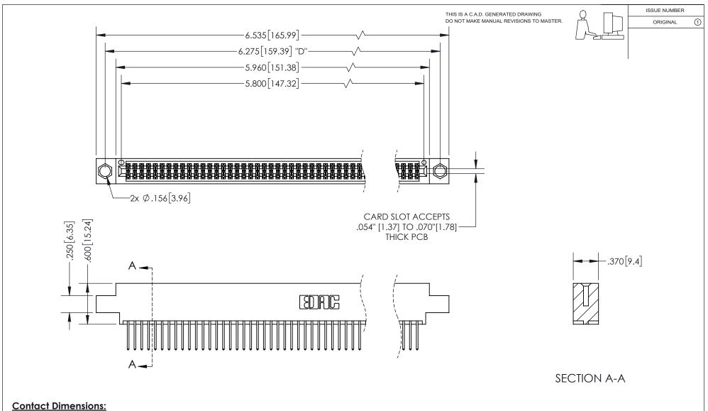
523-P.C. Tail .025 Sq.(0.64 Sq.) - Tail LG=.390(9.91) .100 (2.54) Contact Spacing x .200 (5.08) Row Spacing
