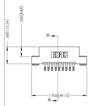
INSULATOR MATERIAL: THERMOPLASTIC POLYESTER, UL 94V-0 CONTACT MATERIAL; COPPER, NICKEL, TIN ALLOY CA-725 CONTACT PLATING: GOLD ON THE MATING AREA, TIN-LEAD
