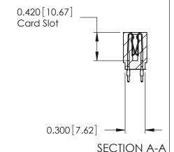
725 Series Ultra-Mate Card Edge Connector - Press Fit
