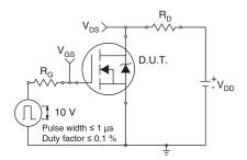
Fig. 13 - Switching Time Test Circuit
