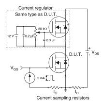
Fig. 18 - Gate Charge Test Circuit
