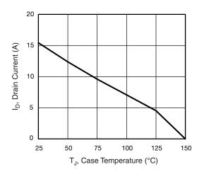
Fig. 10 - Maximum Drain Current vs. Case Temperature
