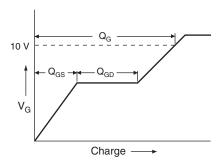
Fig. 17 - Basic Gate Charge Waveform
