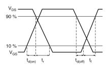
Fig. 14 - Switching Time Waveforms
