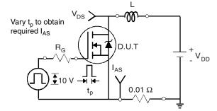
Fig. 15 - Unclamped Inductive Test Circuit
