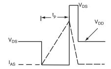
Fig. 16 - Unclamped Inductive Waveforms
