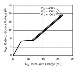
Fig. 7 - Typical Gate Charge vs. Gate-to-Source Voltage
