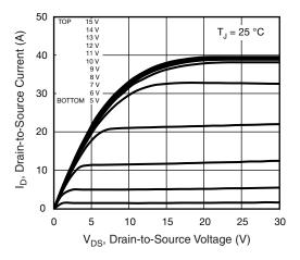
Fig. 1 - Typical Output Characteristics
