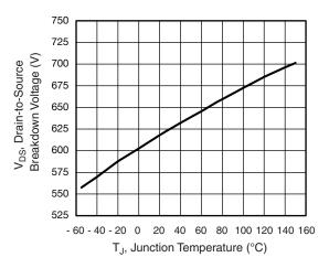
Fig. 11 - Temperature vs. Drain-to-Source Voltage
