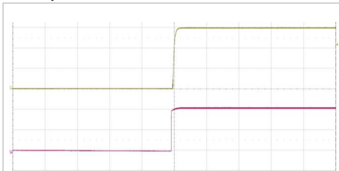
Start-up enabled by connecting V_i at: T_{P1} = +25^{\circ}\text{C} , V_i = 110\text{ V} , I_o = 10\text{ A} resistive load. Top trace: output voltage (5 V/div.). Bottom trace: input voltage (50 V/div.). Time scale: (100 ms/div.).
