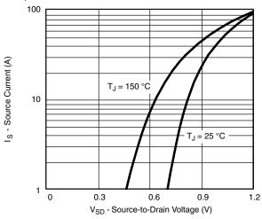
Source-Drain Diode Forward Voltage
