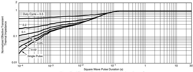
Normalized Thermal Transient Impedance, Junction-to-Case
