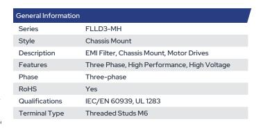
**Specifications** 530 VAC, 305 VAC Voltage AC 50-60 Hz Rated Frequency Rated Current 42 A (50°C) Rated Temperature 50°C Temperature Range -25/+100°C Climate Category 25/100/21 Test Voltage DC (P to P) 2250 VDC Test Voltage DC (P to E) 3000 VDC 15 W (25°C 50 Hz) Power Loss Leakage Current 4.7 mA
