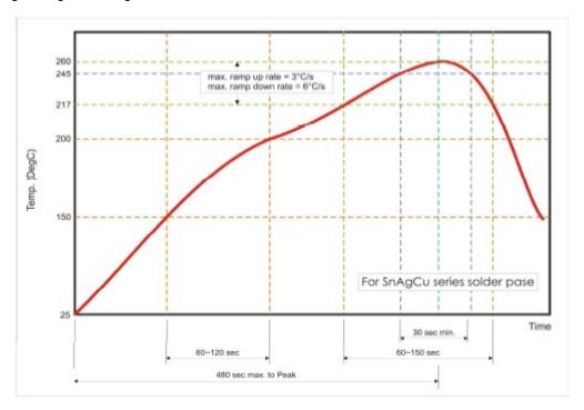
Fig 3. Infrared soldering profile for Chip Resistors WW25
