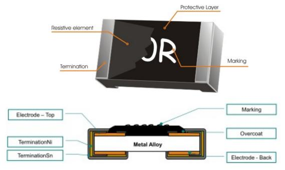
Fig 1. Construction of Chip-R
