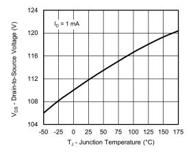
**Drain Source Breakdown vs. Junction Temperature**
