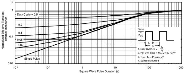
Normalized Thermal Transient Impedance, Junction-to-Ambient
