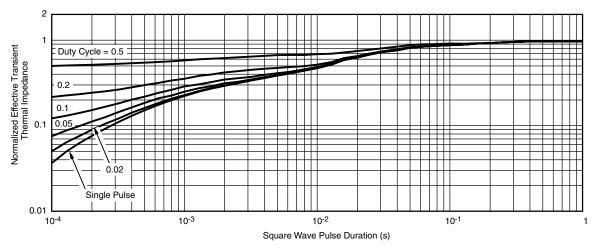
Normalized Thermal Transient Impedance, Junction-to-Case
