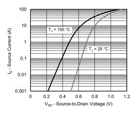
**Source Drain Diode Forward Voltage**
