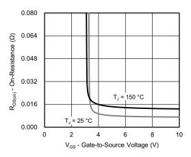
On-Resistance vs. Gate-to-Source Voltage
