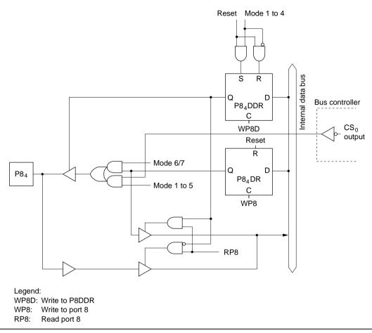
Figure C.8 (c) Port 8 Block Diagram (Pin P8<sub>4</sub>)
