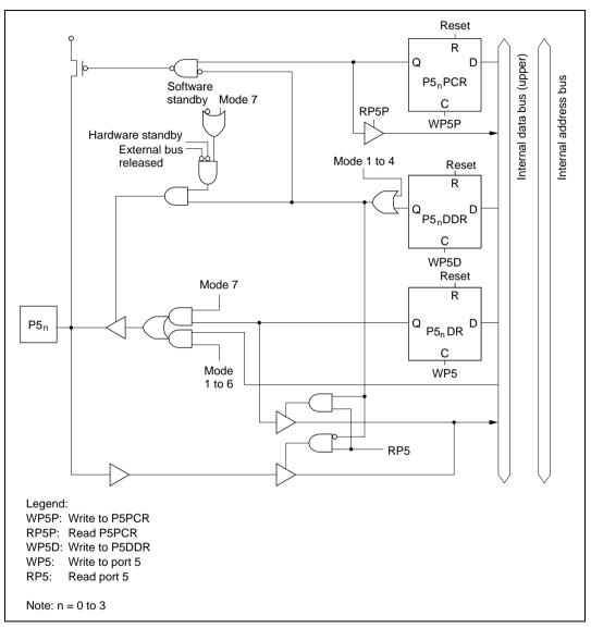
Figure C.5 Port 5 Block Diagram
