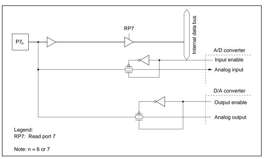
Figure C.7 (b) Port 7 Block Diagram (Pins P7<sub>6</sub>, P7<sub>7</sub>)
