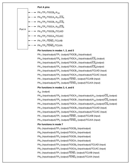
Figure 9.10 Port A Pin Configuration
