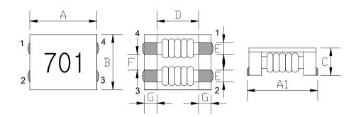
A: 12.0±0.5 mm A1: 12.5±0.5 mm B: 10.8±0.5  $\mathbf{m}\mathbf{m}$ C: 6.4 Max. mm D: 7.0 Typ. mm E: 2.7±0.2 mm F: 2.5±0.2 mm G: 2.5±0.2 mm
