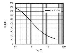
Fig. 2 - Typical Diode Capacitance vs. Reverse Voltage
