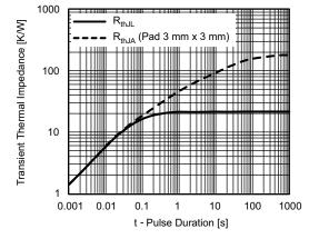
Fig. 5 - Typical Transient Thermal Impedance
