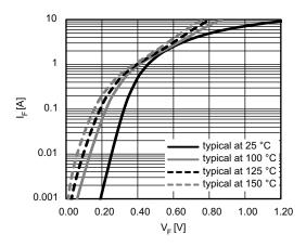
Fig. 1 - Typical Forward Characteristics
