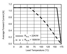
Fig. 4 - Forward Current Derating Curve
