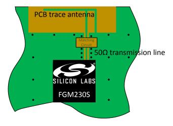
Figure 7.2. FGM230S Implementation with PCB Trace Antenna
