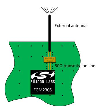
Figure 7.1. FGM230S Implementation with External Antenna
