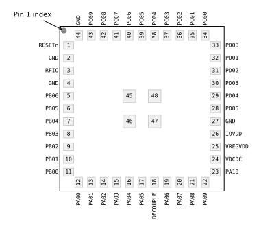
Figure 6.1. FGM230S Module Pinout
