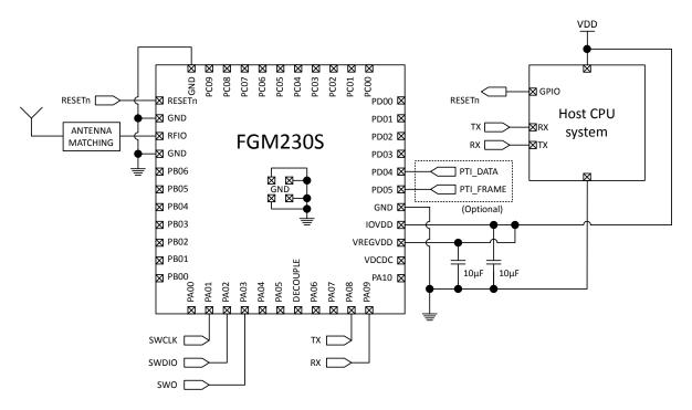
Figure 5.2. Typical FGM230S Host CPU Connections
