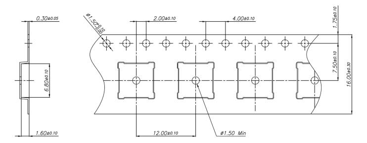
Figure 10.1. Carrier Tape Dimensions
