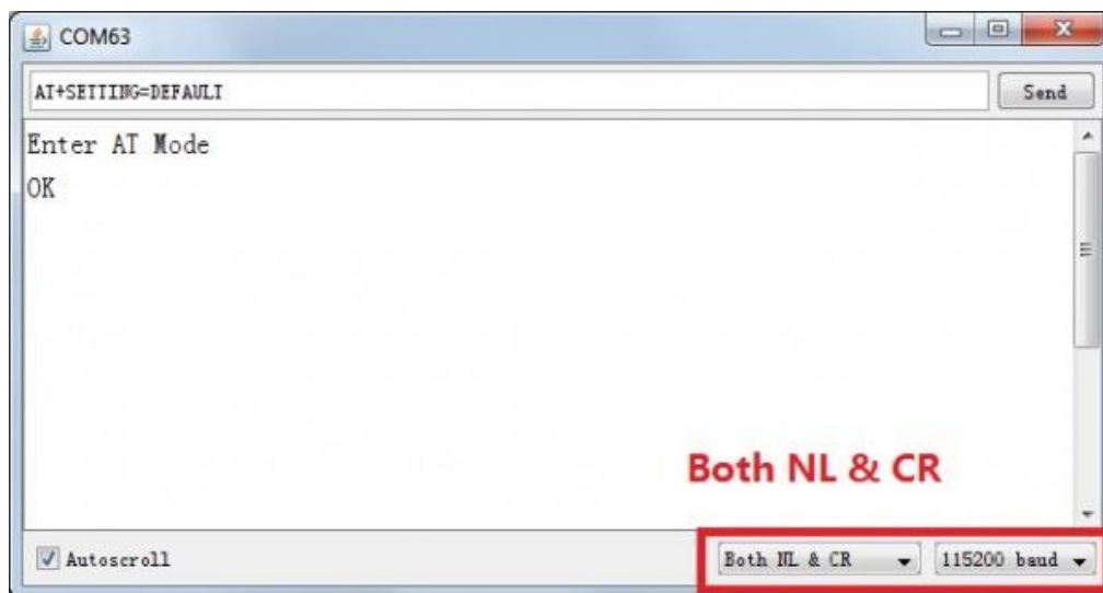
Fig1: enter the AT command, remember selecting the Both NL & CR
