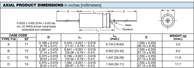
For insulated parts, add 0.015" [0.38 mm] to the diameter. The insulation shall lap over the ends of the capacitor body
