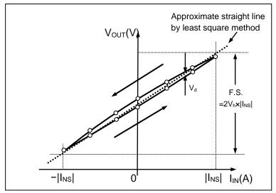
Figure 5. Output characteristics of CQ-2234
