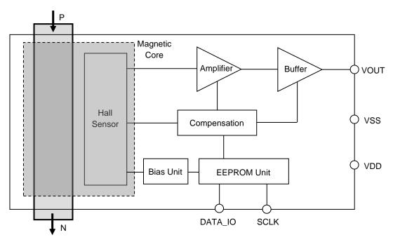
Figure 1. Functional block diagram of CQ-2234
