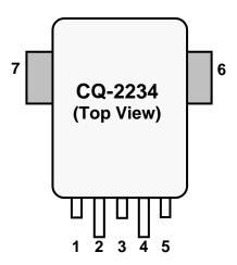
Figure 3. Pin assignment of CQ-2234
