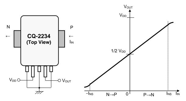
Figure 2. Output characteristics of CQ-2234
