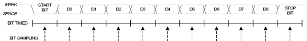
Figure 26.4. 9-Bit UART Timing Diagram
