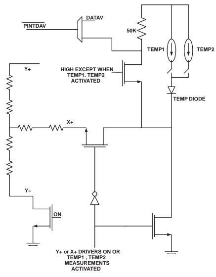
Figure 13. **PINTDAV** Functional Block Diagram
