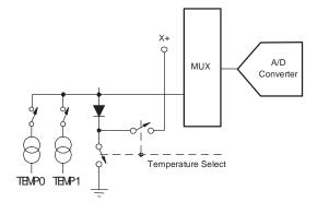
Figure 14. Functional Block Diagram of Temperature Measurement Mode
