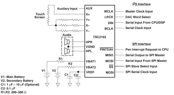
Figure 9. Typical Circuit Configuration
