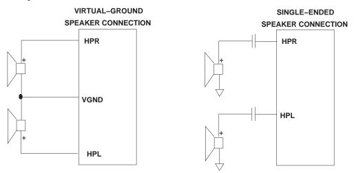
Figure 22. Connection Diagram for DAC Outputs
