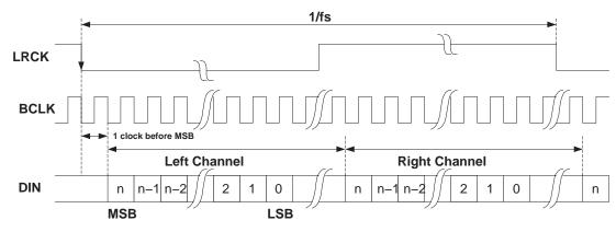
Figure 20. Timing Diagram for I2S Mode
