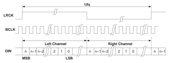
Figure 19. Timing Diagram for Left-Justified Mode
