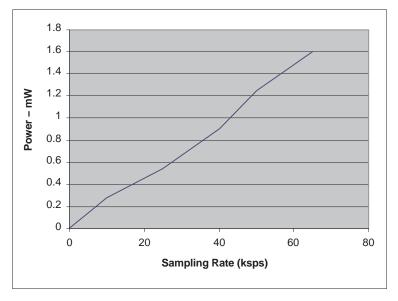
Figure 7. Touch Screen Power Consumption With Speed ( $T_A = 25^{\circ}C$ , External Ref, Host Controlled AUX Conversion, AVDD = 3.3 V)
