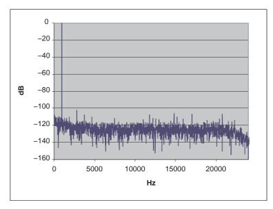
Figure 8. DAC FFT Plot (T<sub>A</sub> = 25°C, 48 ksps, 0 dB, 1 kHz Input, AVDD = 3.3 V, R<sub>L</sub> = 10 k $\Omega$ )
