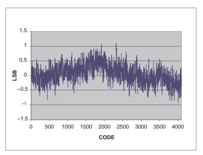
Figure 5. SAR INL (T<sub>A</sub> = 25°C, Internal Ref = 2.5 V, 12 bit, AVDD = 3.3 V)
