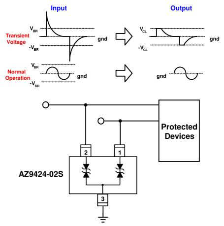
Fig. 1 The ESD protection scheme by using AZ9424-02S.
