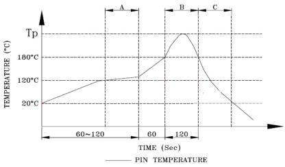
A. Preheating B. Soldering C. Gradual Cooling
