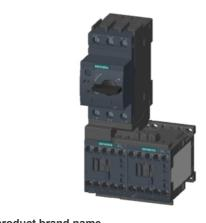
Load feeder fuseless, Reversing duty 400 V AC, Size S00 5.50...8.00 A 230 V AC screw terminal for installation on standard mounting rail Type of coordination 1, lq = 150 kA 1 NC (contactor)
