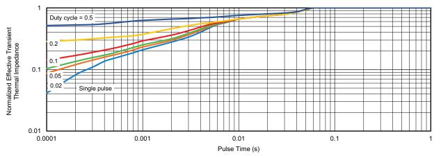
Fig. 12 - Normalized Transient Thermal Impedance, Junction-to-Case
