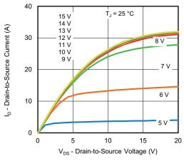
Fig. 1 - Typical Output Characteristics
