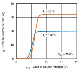
Fig. 3 - Typical Transfer Characteristics
