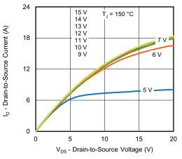
Fig. 2 - Typical Output Characteristics
