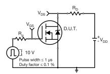
Fig. 13 - Switching Time Test Circuit
