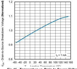
Fig. 11 - Temperature vs. Drain-to-Source Voltage
