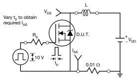
Fig. 15 - Unclamped Inductive Test Circuit
