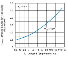
Fig. 4 - Normalized On-Resistance vs. Temperature
