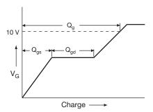
Fig. 17 - Basic Gate Charge Waveform
