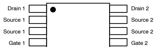
Figure 3. Pinouts for Dual-Die TSSOP
