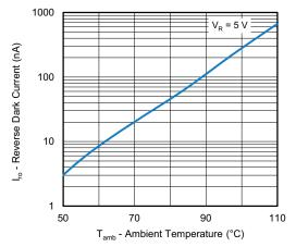
Fig. 1 - Reverse Dark Current vs. Ambient Temperature
