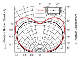
Fig. 6 - Relative Radiant Sensitivity vs. Angular Displacement
