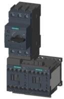
FUSELESS MOTOR STARTER REVERSING OPERATION 600V AC SZ S00 1.8-2.5A 220/240V AC 50/60HZ SCREW CONNECTION FOR SCREW MOUNTING OR 35 MM RAIL-MOUNTING TYPE OF COORDINATION 2 IQ = 150 KA ALSO FULFILLS TYPE OF COORDINATION 1 1NC (PER CONTACTOR)
