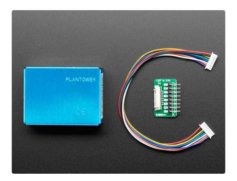
You'll need to hook this up to a microcontroller with UART input (or you could theoretically wire it up to a USB-Serial converter and parse the data on a computer ()) - we have code for both Arduino and CircuitPython. 9600 baud data streams out once per second, you'll get:
