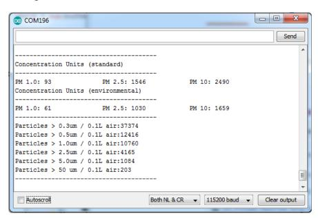
Note that the numbers are very precise looking but we don't believe that they're going to be perfectly accurate, calibration may be necessary!
