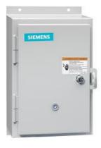
Reversing motor starter, Size 0, Three phase full voltage, Solid-state overload relay, OLR amp range 0.25-1A, Non-combination type, Enclosure type 12, Dust/drip proof for indoors, Standard width enclosure
