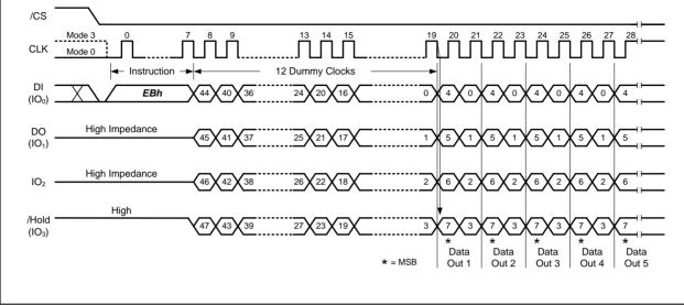
Figure 25b. Fast Read Quad I/O Instruction (Sequential Read Mode, BUF=0)
