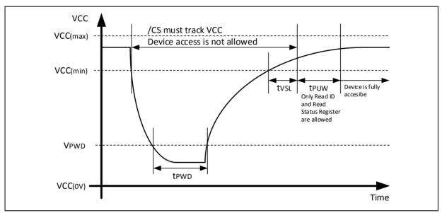
Figure 29. Power-up Timing and Voltage Levels
