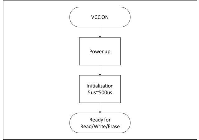
Figure 3. W25N04KV Flash Memory Operation Diagram
