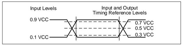
Figure 31. AC Measurement I/O Waveform
