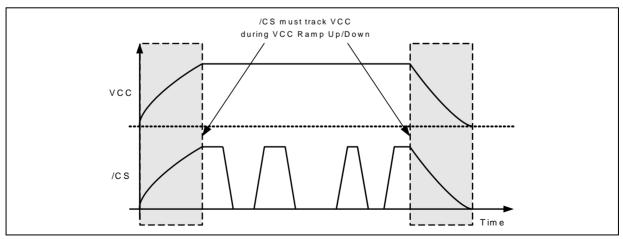
Figure 30. Power-up, Power-Down Requirement
