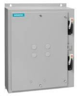
Duplex starter w/o alternator Size 0 Three phase full voltage Solid-state overload relay OLR amp range 0.75-3.4A 24VAC 50-60Hz Coil Combination type Two 30A disconnect switches Encl NEMA type 4X 304 S. Steel Water/dust tight non-corrosive
